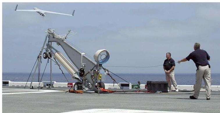
*Fig. 1.1.46. Lansator pneumatic*
